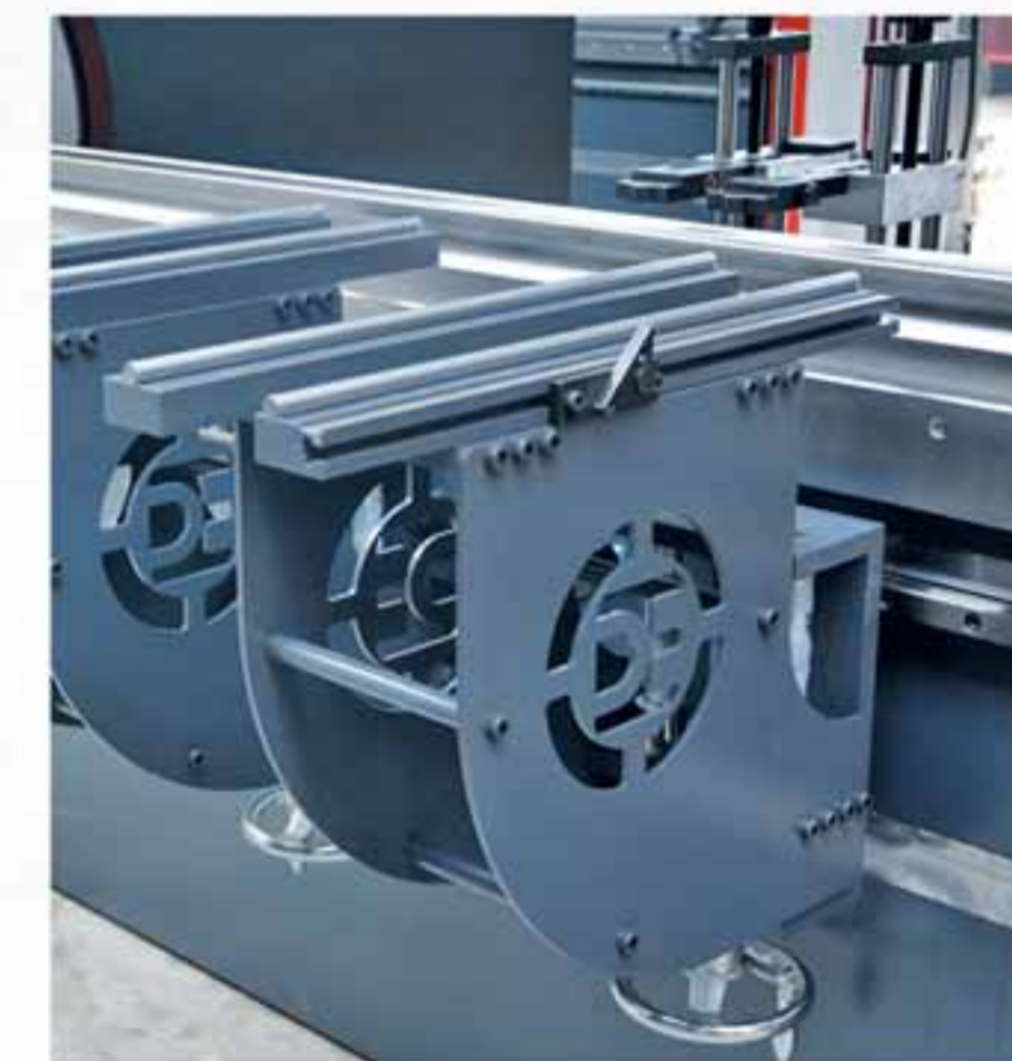
Linear Guided Stronger Front Supports (Above 175 tons machine)
